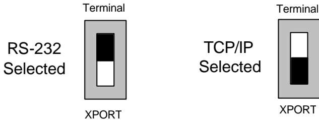
Figure 7. RS-232 /TCP/IP connection selector switch (V2 board)
