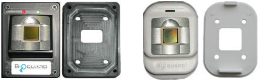
Figure 14. Series I Sensor (left) and Series II Sensor (right) and locations of relevant fixing holes
